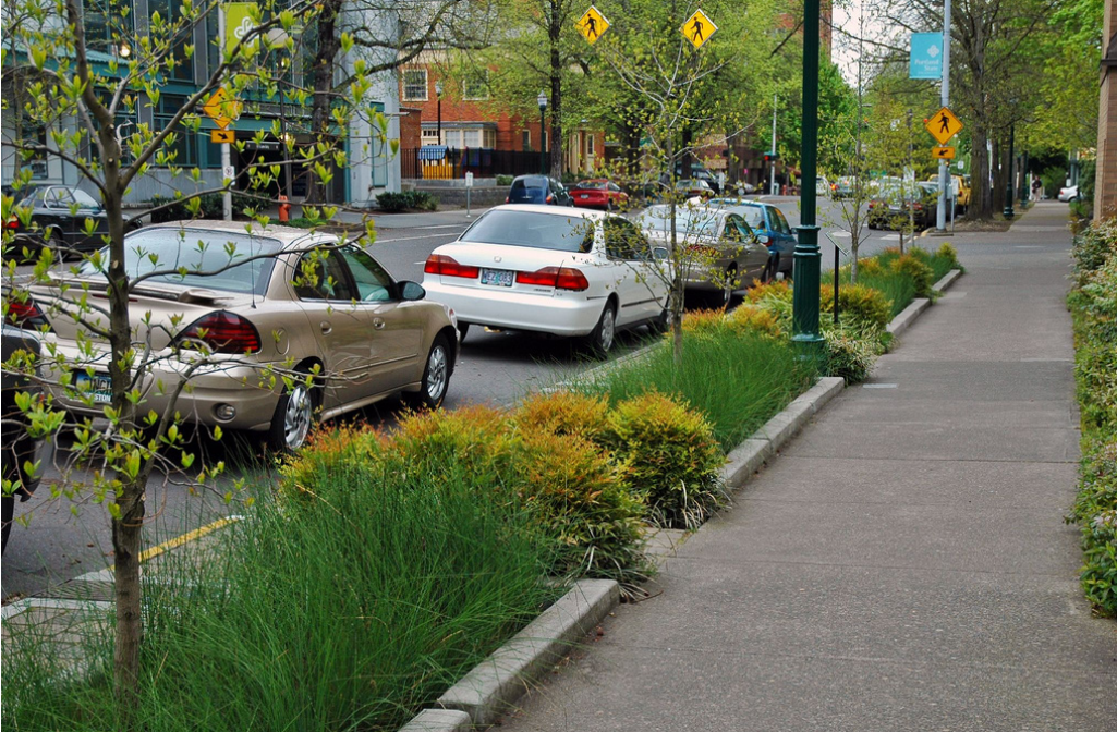
12th Avenue Green Street featuring bioswales near the Portland State University campus ( http://flickr.com/photos/sitephocus/2629874914/ )
