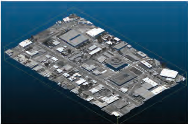
POINT CLOUD DATA FROM AERIAL LIDAR SCAN Source: Washington State Department of Natural Resources
