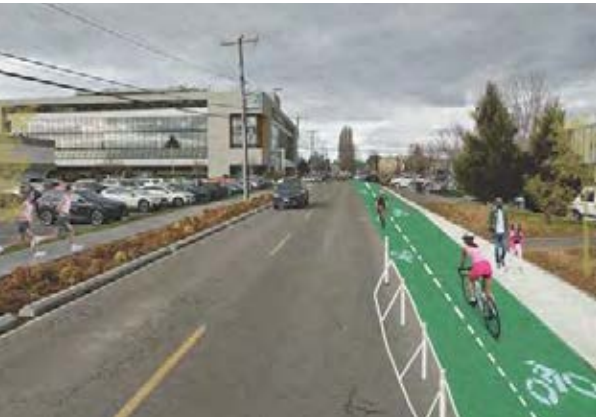
6TH AVENUE SOUTH BIKE IMPROVEMENTS UTILIZING EXISTING ON-STREET PARKING SPACE FOR A TWO-WAY BIKE LANE.
