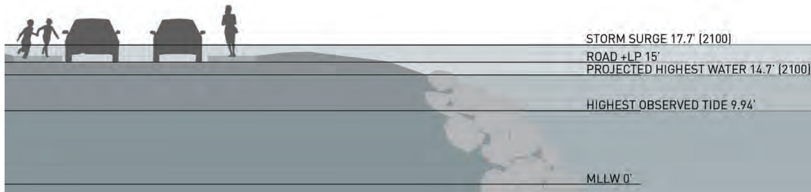
FIGURE 4: Section of projected sea level rise impacts on the Waterfront District, informed by the Bellingham Waterfront District Sub-Area Plan 2019
