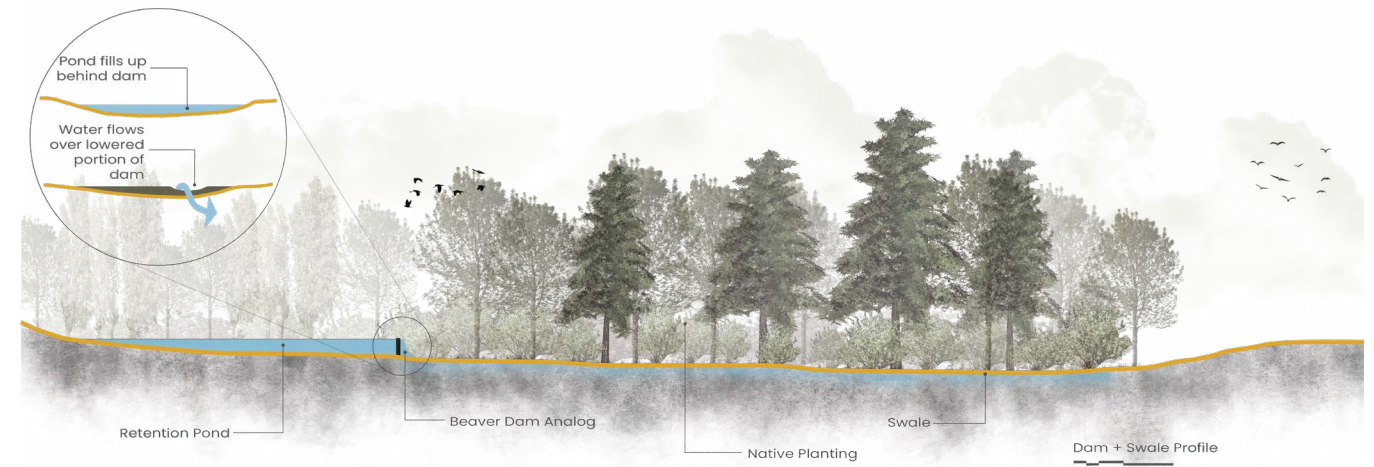
C: North-South site section through Retention Pond, Beaver Dam Analog, and Native Planting Swale. Graphic by Emma Petersen
