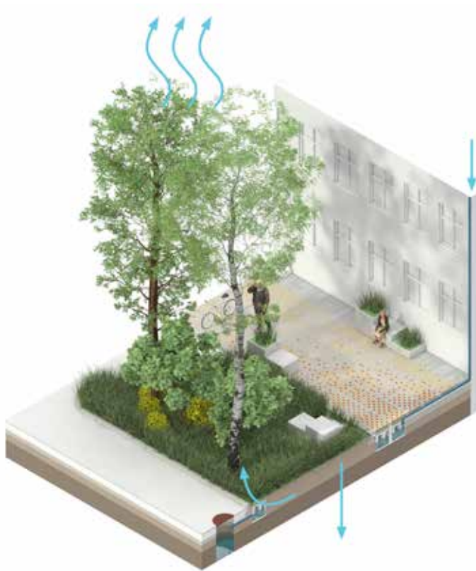
Collecting rain water from roof and pavement and using it in various ways
