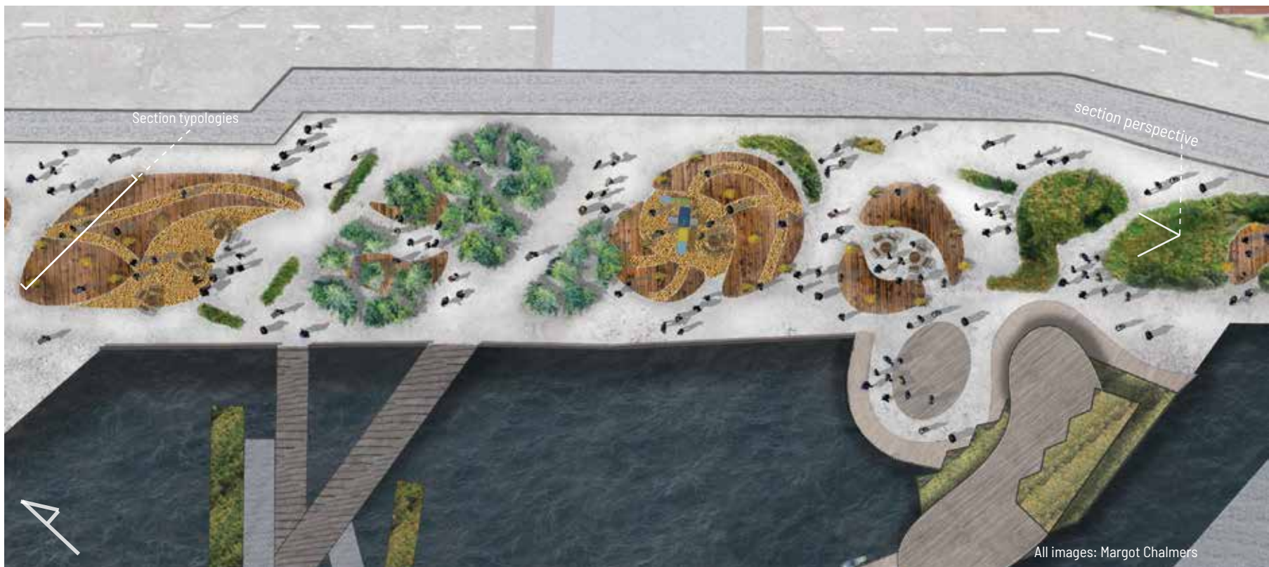
(Above) Plan Detail: This segment of the plan depicts how the Dunescape connects and functions with the community center and boardwalk.
